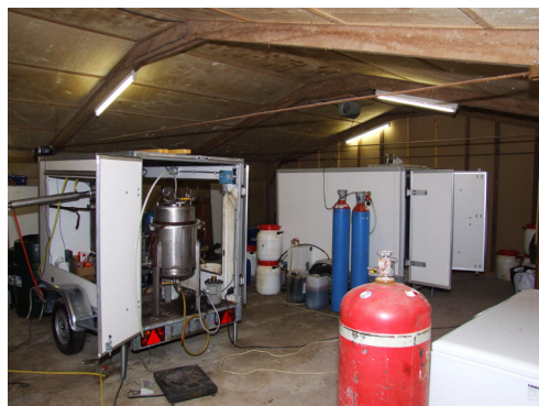
Mobile MDMA production unit with pressure reaction vessel and distillation (front, left); a mobile tableting unit (back, right). Photo: Europol.
